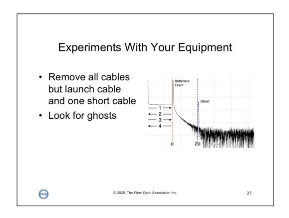
Set up your OTDR and launch cable only. Attach a fairly short cable to the launch cable and take a trace. Do you see more than one reflection from the connection and the end of the short cable? How do you know those are ghosts.
