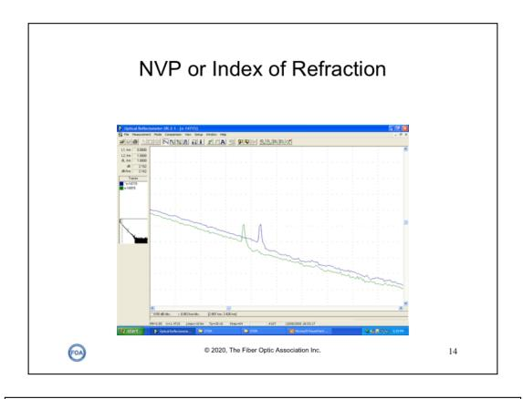
The index of refraction of the fiber is a measure of how fast light travels in the fiber - the nominal velocity of propagation. If we change the index of refraction, it changes the calibration of the OTDR distance scale, so we need to know it to calibrate the measured length of the fiber.
