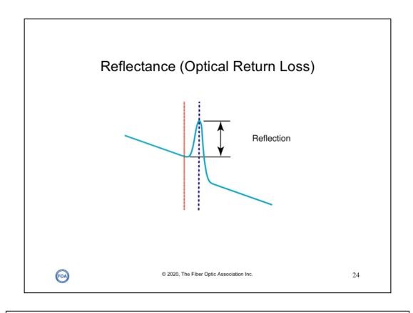
connector or splice (usually a mechanical splice.) This is a complicated process involving the baseline of the OTDR, backscatter level and power in the reflected peak. Like all backscatter measurements, it has a fairly high measurement uncertainty, but has the advantage of showing where reflective events are located so they can be corrected if necessary.
