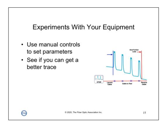
Using the manual controls for setup of the OTDR parameters, select the proper wavelength, the shortest range that allows you to test your simulated cable plant, the shortest test pulse and minimal averaging.
