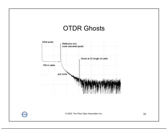
If you are testing short cables with highly reflective connectors, you will likely encounter "ghosts." These are caused by the reflected light from the far end connector reflecting back and forth in the fiber until it is attenuated to the noise level.
