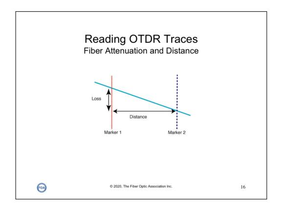
The OTDR display is usually called a "trace." It includes the backscatter trace from the fiber under test, several "markers" which can be moved along the trace to pinpoint the places on the trace from which measurements are made, and usually a number of digital displays of distance and loss. The easiest way to understand what you see is to consider the figure below, a simple trace from which we will measure the length and attenuation coefficient of the fiber.
