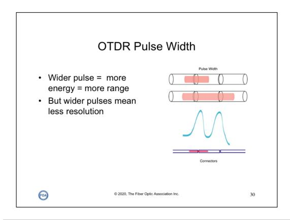
The amount of light scattered back to the OTDR is proportional to the backscatter of the fiber, peak power of the OTDR test pulse and the length of the pulse sent out. If you need more backscattered light to get good measurements, you can increase the pulse peak power or pulse width. Most OTDRs allow you to change the pulse width and some also can set pulse power higher at longer ranges.
