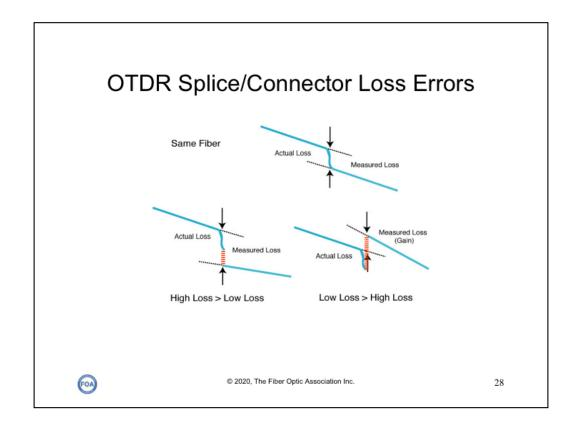
Another problem that occurs is a function of the backscatter coefficient, the amount of light from the outgoing test pulse that is scattered back toward the OTDR. The OTDR looks at the returning signal and calculates loss based on the declining amount of light it sees coming back.
