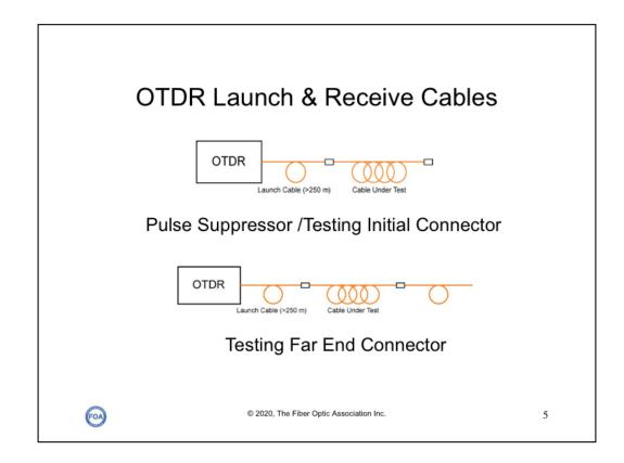
OTDRs should always be used with a launch cable often called a "pulse suppresser" cable, which doesn't suppress pulses, but simply gives the OTDR time to recuperate before you start looking at the fiber in the cable plant you want to test. *Do not ever use an OTDR without this launch cable!*
