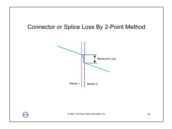
To measure splice loss, move the two markers close to the splice to be measured, having each about the same distance from the center of the splice. The splice won't look as neat as this, with the instrument resolution and noise making the trace less sharp looking, as you will see later on. The OTDR will calculate the dB loss between the two markers, giving you a loss reading in dB.
