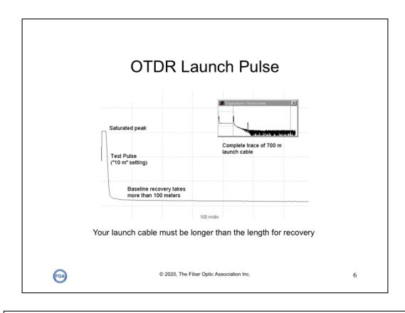
Since so little of the light comes back to the OTDR for analysis, the OTDR receiver circuit must be very sensitive. That means that big reflections, which may be one percent of the outgoing signal, will saturate the receiver, or overload it. Once saturated, the receiver requires some time to recover, and until it does, the trace is unreliable for measurement as shown.
