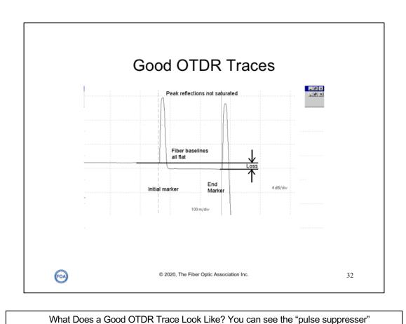
launch cable, the first fiber out from the OTDR, allows time for the OTDR to recover from the initial pulse. Note the fibers are all straight lines between "events", as splices and connectors are called in OTDR jargon. Markers for loss measurements should always be set far enough on either side of an event to be on the straight part of the fiber trace. If there is any curve, it is likely caused by the resolution of the OTDR or recovery from an overload.
