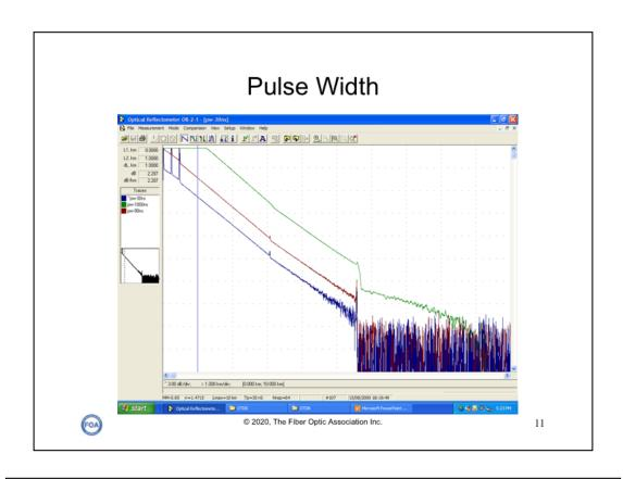
Widening the pulse width means there is more energy - more signal - in each pulse. You can see the effect above, as the lower (blue) pulse is the shortest with the best resolution but has the most noise. As we go to wider pulses, you get less noise and more range, but less resolution. In the top trace, we have lots of power, but the events are spread out so much to be hard to distinguish.
