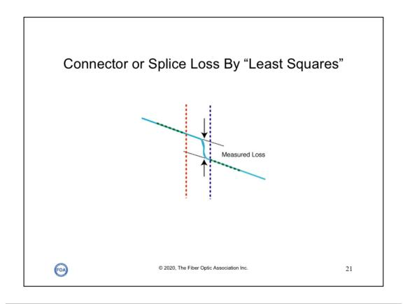
If you noticed, the markers are separated by some distance, which includes the loss of some fiber on either side of the actual connector or splice. Most OTDRs will calculate the loss for you by extrapolating the fiber traces on both sides of the event and calculating the loss without any influence from the fiber length. The mathematical method uses is called "Least Squares Approximation", hence the term "LSA" used by many OTDRs in their display and setup menus.
