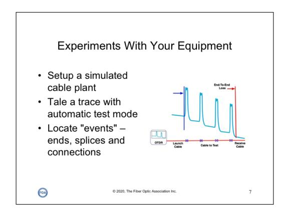
If you have an OTDR and some long-ish fiber optic cables, here are some experiments to perform. Use connectors and splices to connect the cables.
