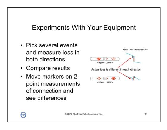
Using the same setup, measure several connection or splice losses with LSA methods. Then reverse the test setup for the "cable under test" so you can test the same connections or splices in the opposite direction. (Be sure to not disconnect the connections your are testing so you have the same setup to compare the same connections or splices in opposite directions.) How close do they agree?
