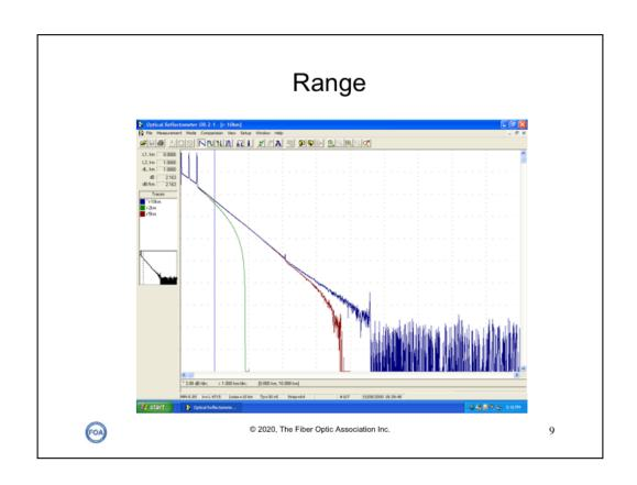
The range should be set at two times the length of the cable to prevent confusing the OTDR. Shown here are three traces of a 5.2 km link taken at ranges of 2, 5 and 10 km. Note the distortions on the 2 and 5 km traces.
