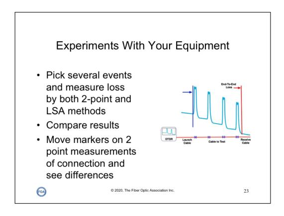
Using the same setup as in Lesson 1, measure several connection or splice losses with both 2-point and LSA methods. How close do they agree?
